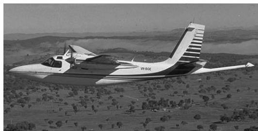
**Figure 21** An Aero-Commander Shrike aircraft fitted with a magnetometer in a tail stinger for aeromagnetic surveying. Courtesy of Geoscience Australia.
